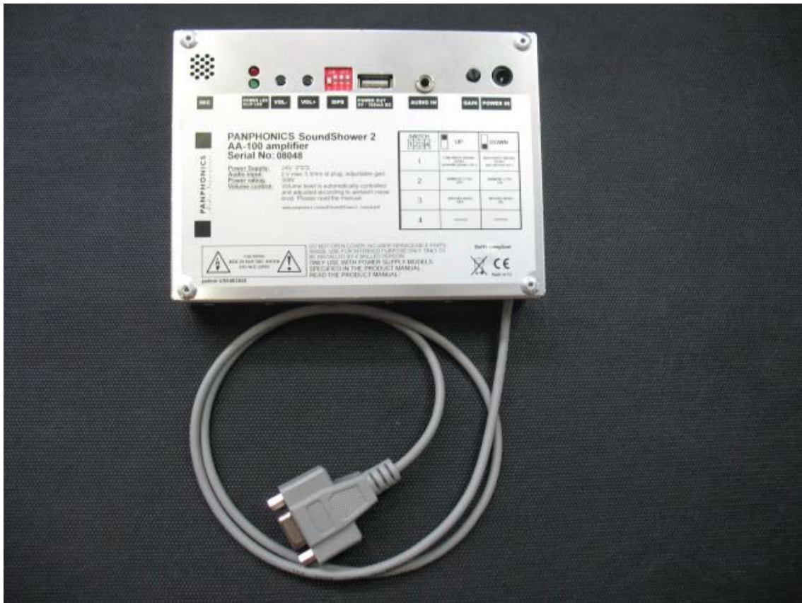
Figure 16. AA100E amplifier back plate and 0.80 m cable with d-connector
